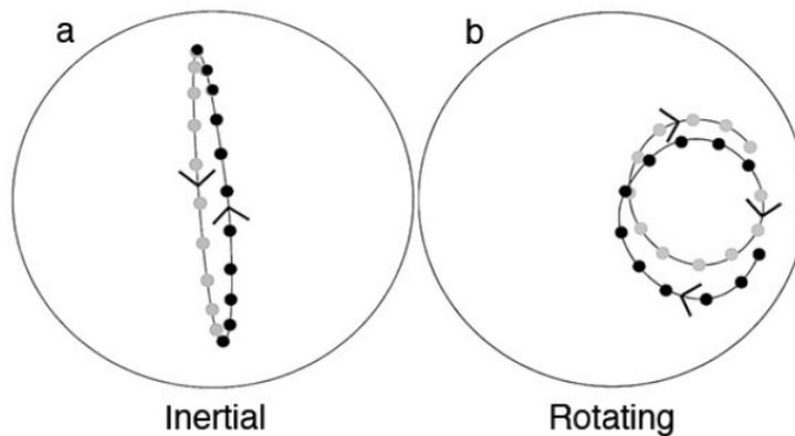
Figure 6.14: Trajectory of the puck on the rotating parabolic surface during one rotation period of the table  $\frac{2\pi}{\Omega}$  in (a) the inertial frame and (b) the rotating frame of reference. The parabola is rotating in an anticlockwise (cyclonic) sense.
