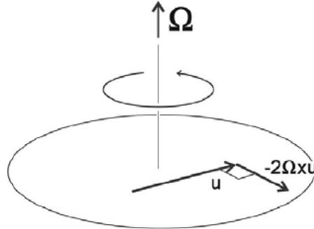
Figure 6.10: A fluid parcel moving with velocity  $u_{rot}$  in a rotating frame experiences a Coriolis acceleration  $-2\vec{\Omega} \times u_{rot}$ , directed ‘to the right’ of  $u_{rot}$  if, as here,  $\vec{\Omega}$  is directed upwards, corresponding to anticlockwise rotation.
