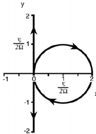
Figure 6.15: Theoretical trajectory of the puck during one complete rotation period of the table,  $\frac{2\pi}{\Omega}$ , in GFD Lab V in the inertial frame (straight line) and in the rotating frame (circle). We launch the puck from the origin of our coordinate system  $x(0) = 0; y(0) = 0$  (chosen to be the center of the rotating parabola) with speed  $u(0) = 0; v(0) = v_o$ . The horizontal axes are in units of  $\frac{v_o}{2\Omega}$ . Observed trajectories are shown in Fig.6.14.
