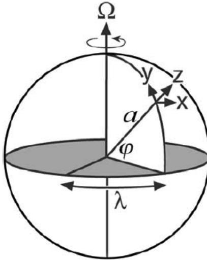
Figure 6.19: At latitude  $\varphi$ , longitude,  $\lambda$ , we define a local coordinate system such that the three coordinates in the  $(x, y, z)$  directions point (eastward, northward, upward):  $dx = a \cos \varphi d\lambda$ ;  $dy = a d\varphi$ ;  $dz = dz$  where  $a$  is the radius of the earth. The velocity is  $\mathbf{u} = (u, v, w)$  in the directions  $(x, y, z)$ . See also Section 13.2.3.
