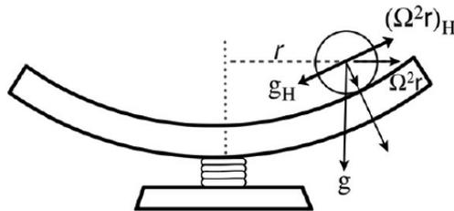
Figure 6.12: If a parabola of the form given by Eq.(6.33) is spun at rate  $\Omega$ , then a ball carefully placed on it at rest does not fall in to the center but remains at rest: gravity resolved parallel to the surface,  $g_H$ , is exactly balanced by centrifugal accelerations resolved parallel to the surface,  $(\Omega^2 r)_H$ .
