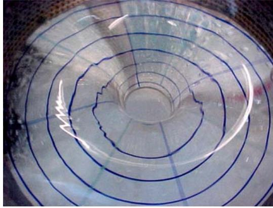
Figure 6.7: The free surface of the radial inflow experiment, in the case when the apparatus is rotated anticyclonically. The curved surface provides a pressure gradient force directed inwards that is balanced by an outward centrifugal force due to the anticlockwise circulation of the spiraling flow.
