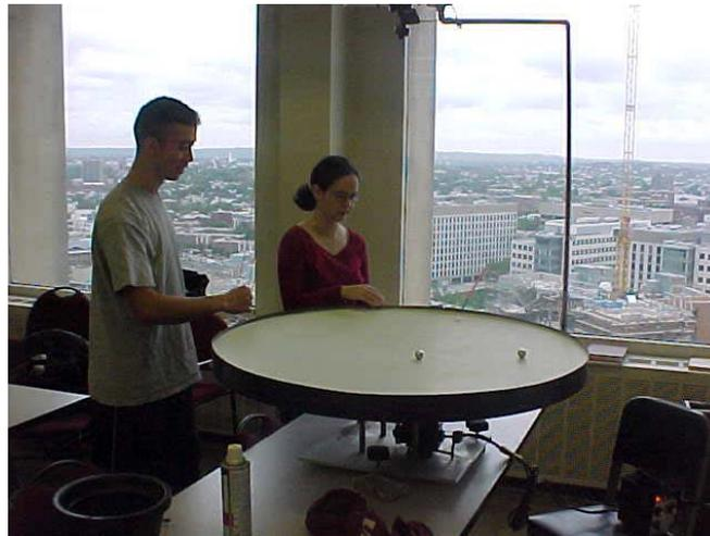
Figure 6.13: Studying the trajectories of ball bearings on a rotating parabola. A co-rotating camera views and records the scene from above.
