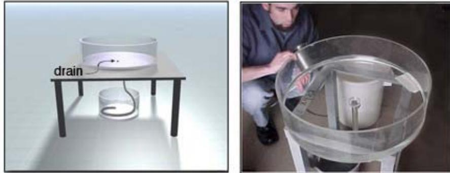
Figure 6.20: A leveled cylinder is filled with water, covered by a lid and left standing for several days. Attached to the small hole at the center of the cylinder is a hose (also filled with water and stopped by a rubber bung) which hangs down in to a pail of water. On releasing the bung the water flows out and, according to theory, should acquire a spin which has the same sense as that of the Earth.
