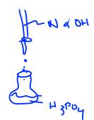
1. Your lab TF gives you a 50.0 mL sample of a phosphoric acid solution of unknown concentration. You are asked to determine the concentration of this solution by titrating it with a 0.731-molar sodium hydroxide solution. 9431mor
