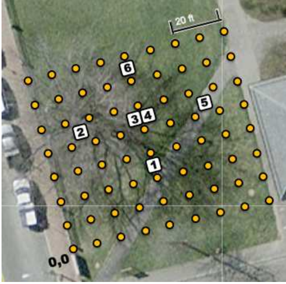
Figure 6: A satellite image of the experiment landscape. Broadcasting motes are denoted by numbered squares and measurement points (where the receiver is placed) are denoted as orange circles. The origin of the measurement grid is in the lower left corner.
