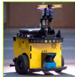
Pioneer robot with stereo cameras, sonar ring, and LIDAR
