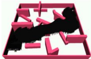
Figure 1b: A nonholonomic planning problem that involves a car pulling three trailers. There are seven degrees of freedom.
